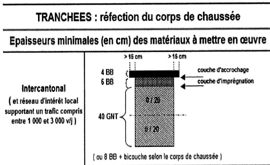
**BB – Béton Bitumineux GB – Grave Bitume GNT – Grave Non Traité**
